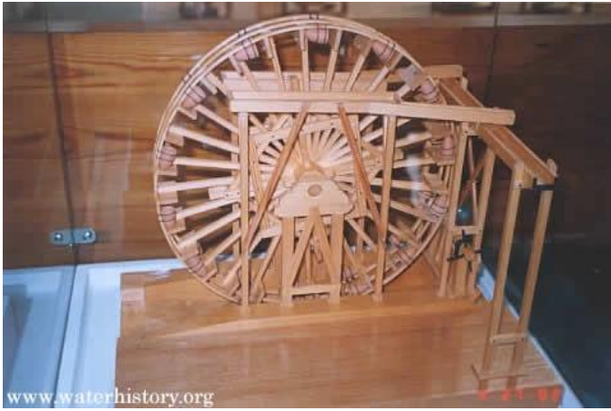
Figure 2.3: A noria, buckets attached to a waterwheel, was another device used to lift water.[27]
